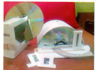
NATIONAL WINNER. The improvised spectroscopy set is specifically designed to measure the wavelength of a specific spectrum of visible light.
